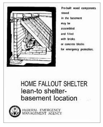
An effective fallout shelter constructed in a basement may reduce your radiation exposure 100-200+ fold. Thus, if the initial radiation intensity outside was 500 R/hr (fatal in one hour), the basement shelter occupants might only experience 5 R/hr or even less, which is survivable, as the radiation intensity will be decreasing with every passing hour.
