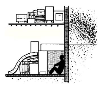
As cramped as that table space fallout shelter might seem, the vital shielding provided by simply moving some mass into place could be the difference between exposure to a lethal dose of radiation and the survival of your family.
